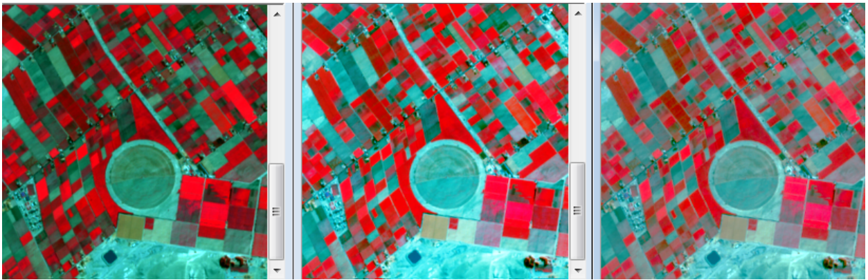
Linear, equal area and Gaussian stretches are illustrated in figure above left to right.
