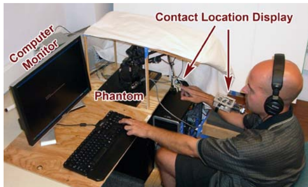
Figure 11. Experiment test setup (cover pulled back for clarity)
