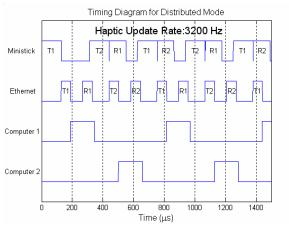
Figure 7: Timing diagram for distributed mode operation running at 3200 Hz.
