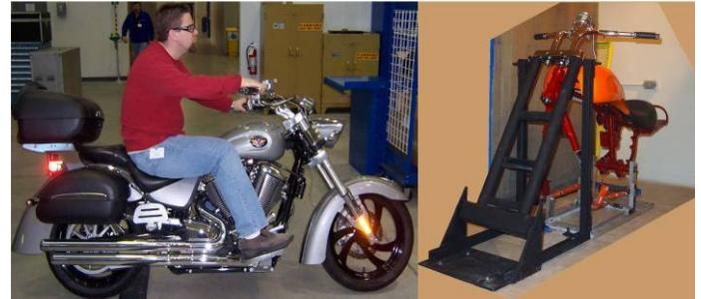
Figure 1. Actual motorcycle sitting posture (left) and test apparatus assembled in our laboratory (right).
