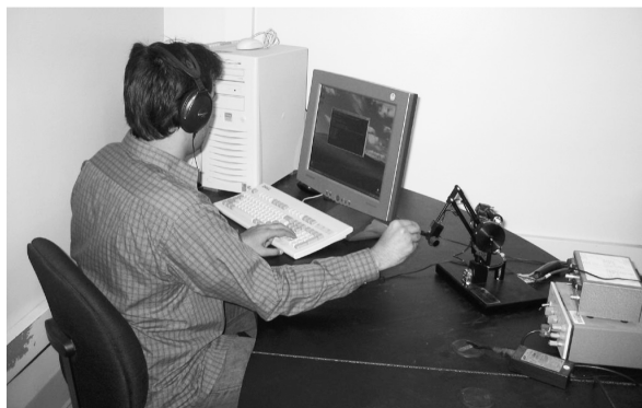
Figure 9. Experimental setup. The participant stroked the virtual haptic textured surface laterally with the right hand. Only text information was available on the computer monitor to indicate the current trial number and to prompt the participant with the response codes.
