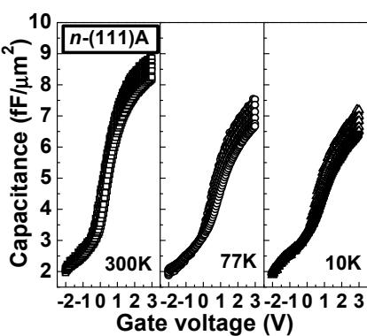
Fig. 8 C-V of Ni/8nm- $\text{Al}_2\text{O}_3$ /n-GaAs(111)A measured at 300K, 77K, 10K. The small drop of the accumulation capacitance is caused by reduction of accumulation charge at low temperatures.
