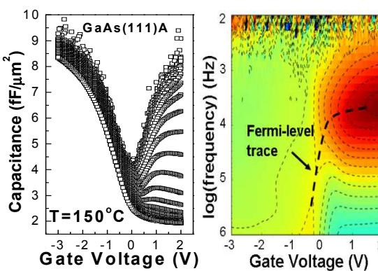
Fig. 14  $C$ - $V$  plot of Ni/8nm-Al<sub>2</sub>O<sub>3</sub>/p-GaAs(111)A at 150°C (left). It shows clear inversion characteristics. The corresponding  $G$ - $V$  plot from 100Hz to 1MHz (right) shows the Fermi-level trace turns to be independent of frequency at 10 KHz, demonstrating real minority carrier (electron) response from inversion.
