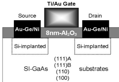
Fig. 1 Schematic view of an inversion GaAs NMOSFET with an ALD  $\text{Al}_2\text{O}_3$  gate dielectric.
