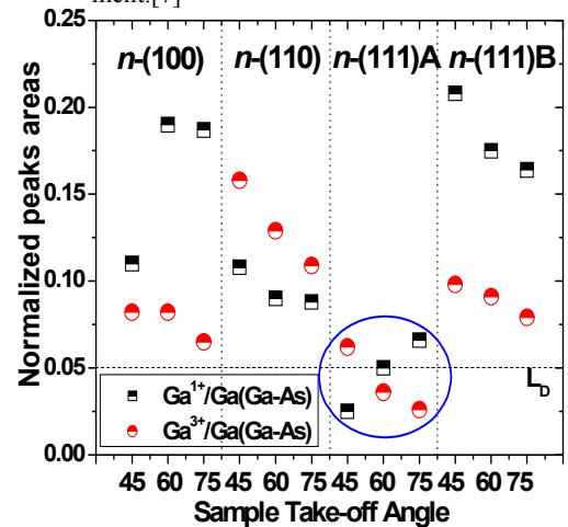
Fig. 18 Ga 2p XPS peak area ratios for various GaAs surface orientations and take-off angles. The GaAs(111)A surface has minimal Ga-oxide formation compared to the other orientations.  $L_D$  notes the detection limit. This correlates with the Fermi-level unpinning on GaAs (111)A from surface analysis.
