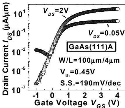
Fig. 5 Transfer characteristic of 4 $\mu\text{m}$  gate length NMOSFET on GaAs(111)A.  $I_{on}/I_{off}$  (@  $V_{DS}=2\text{V}$ ) is about  $1.28 \times 10^4$ .
