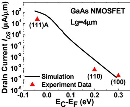
Fig. 10 Simulated drain current as a function of Fermi-level location  $E_F$  relative to the conduction band edge  $E_C$ . The experimental data (in Table 2) follows the simulation line well, showing the extracted ( $E_C - E_F$ ) in Table 2 is valid.
