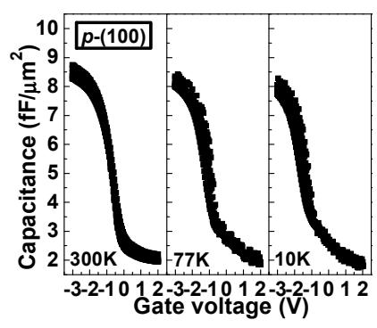
Fig. 12 C-V of Ni/8nm-Al<sub>2</sub>O<sub>3</sub>/p-GaAs(100) measured at 300K, 77K, 10K. Unlike that on n-GaAs(111)A, there is only a small drop of the accumulation capacitance. This indicates that the Fermi-level is not pinned when moving towards the valence band edge  $E_V$ .
