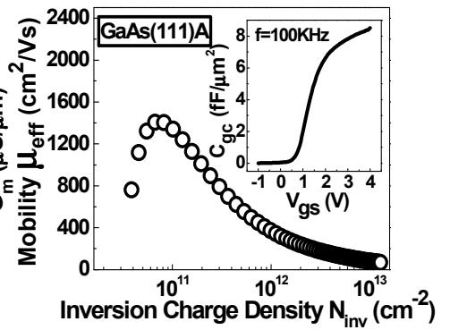
Fig. 7 Effective mobility  $\mu_{eff}$  from 20 $\mu\text{m}$  gate length NMOSFET on GaAs(111)A. The peak electron effective mobility is  $1402 \text{ cm}^2/\text{Vs}$ .
