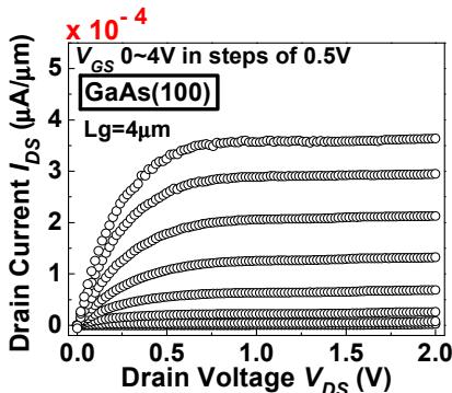
Fig. 2 Output characteristic ( $I_{DS} \sim V_{DS}$ ) for  $\text{Al}_2\text{O}_3/\text{GaAs}(100)$  NMOSFET with 4 $\mu\text{m}$  gate length. The maximum drain current is  $3.5 \times 10^{-4} \mu\text{A}/\mu\text{m}$ .
