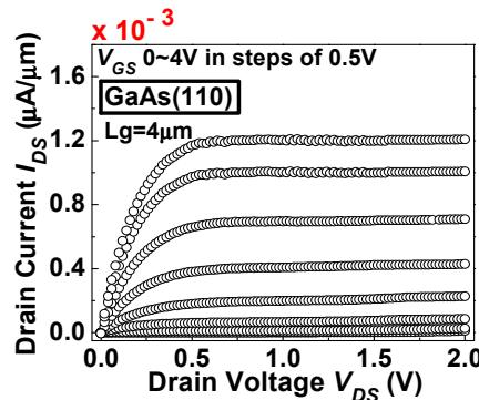
Fig. 3 Output characteristic ( $I_{DS} \sim V_{DS}$ ) for  $\text{Al}_2\text{O}_3/\text{GaAs}(110)$  NMOSFET with 4 $\mu\text{m}$  gate length. The maximum drain current is  $1.2 \times 10^{-3} \mu\text{A}/\mu\text{m}$ .
