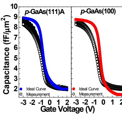
Fig. 13 Ideal high-frequency C-V plots at 27°C. On p-GaAs(111)A, the ideal curve fits very well at both accumulation and inversion sides, demonstrating that Fermi-level can move across the whole band gap. On p-GaAs(100), there is a discrepancy at inversion side, indicating the Fermi-level cannot reach strong inversion.
