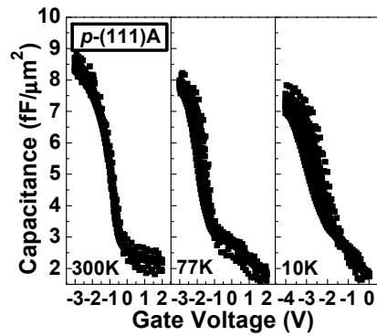
Fig. 11 C-V of Ni/8nm-Al<sub>2</sub>O<sub>3</sub>/p-GaAs(111)A measured at 300K, 77K, 10K. Similar to that on n-GaAs(111)A, there is a small drop of the accumulation capacitance, which is caused by the reduction of accumulation charges at low temperatures.
