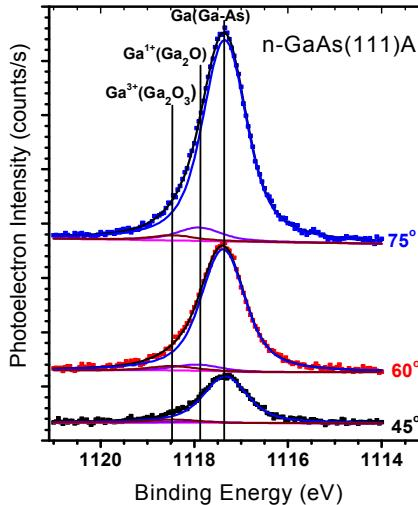
Fig. 16 XPS spectra of Ga 2p region at different take-off angles. Ga-oxides are near the detection limit for GaAs(111)A surface. More Ga-oxides are detected on (111)B, (110) and (100) surfaces.
