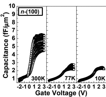
Fig. 9 C-V of Ni/8nm- $\text{Al}_2\text{O}_3$ /n-GaAs(100) measured at 300K, 77K, 10K. The significant drop of the accumulation capacitance is caused by the partial Fermi-level pinning at a certain location in the band-gap.
