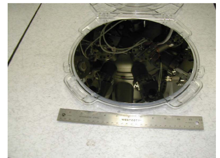
Fig. 16 SrTiO 3 single crystalline film was grown on 300 mm Si substrate by MBE as shown in the picture. The length of the ruler in the picture is 12 inch. The shining SrTiO 3 surface reflects the part of MBE system in which the film was grown.
