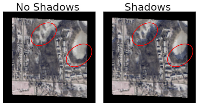
Fig. 9. Example of shadow rendering on OMA 374. Results of rendered images without shadow mask (left) and with shadow mask (right). Regions circled in red contain shadows that are not rendered until after applying the shadow mask.
