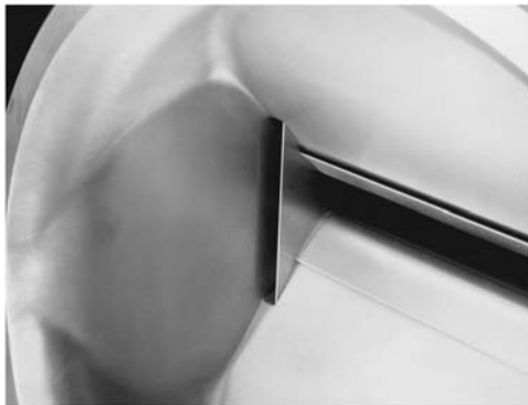
Fig. 6 Bleed slots in subsonic approach to throat of Mach-3.5 quiet nozzle.
