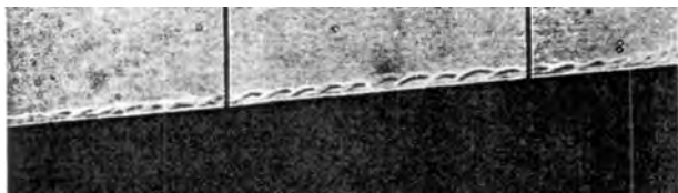
Figure 5: Shadowgraph of Second-Mode Instabilities on a Cone in Air. Zero Angle of Attack, No Blowing. From Ref. [15, Fig. 1a]
