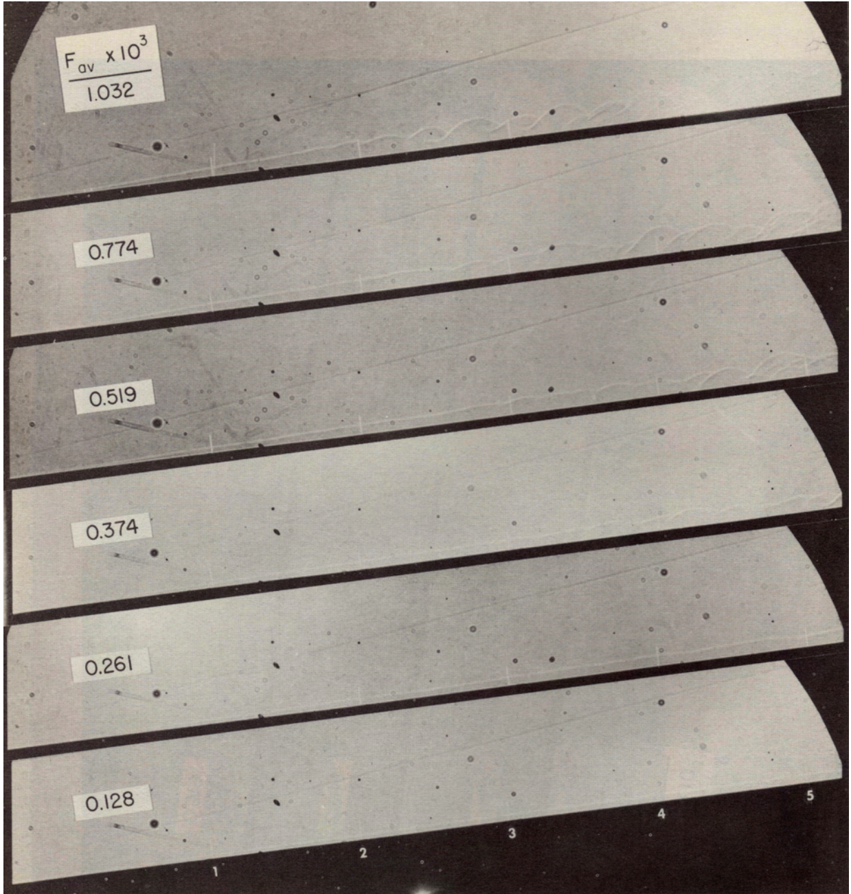
Figure 3: Shadowgraph of Instabilities with Helium Blown into Air. From Ref. [11, Fig. 3d]
