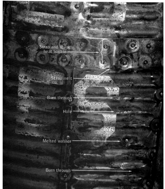
Fig. 24 Closeup of reentry heating damage on the Gemini II spacecraft. From [40].
