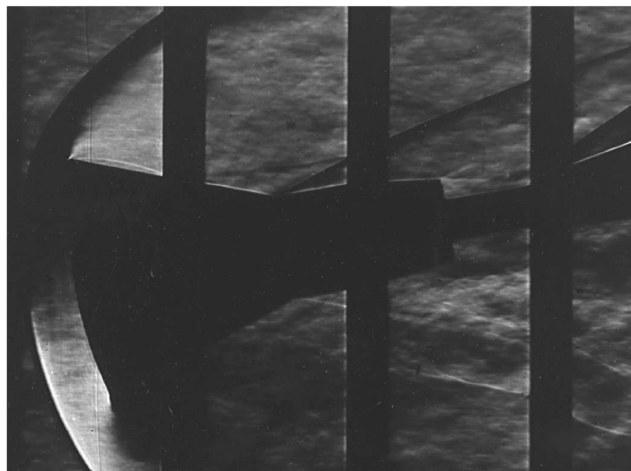
Fig. 27 Schlieren photographs of Gemini reentry configuration at Mach 3.51 and \alpha = -10 deg. Rescaled from Fig. 5a in [46].
