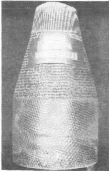
Figure 9: Side View of Laminar-Ablated FWPF Nosetip. From Ref. [55, Fig. 77]
