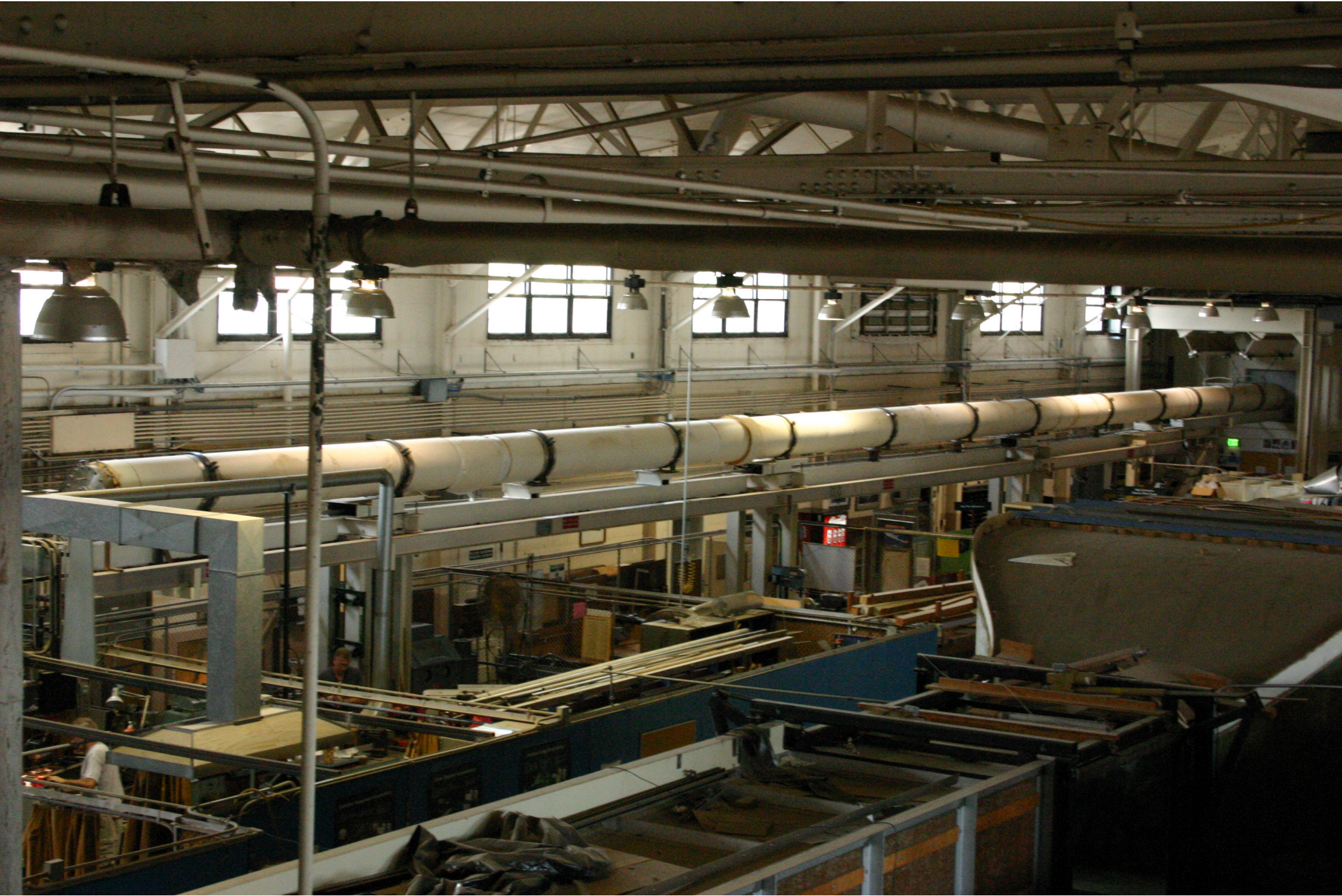
Driver Tube of Mach-6 Quiet Tunnel at Purdue. 120-ft. long by 18-inch diameter, stainless steel.
