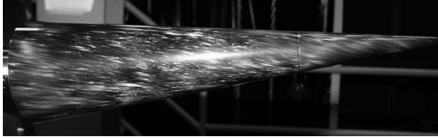
Figure 17: Oil-Flow Image of Streamlines on a Cone at Angle of Attack
