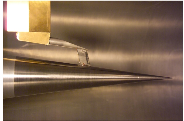
Figure 38: Hot wire in boundary layer of 7 degree blunt cone
