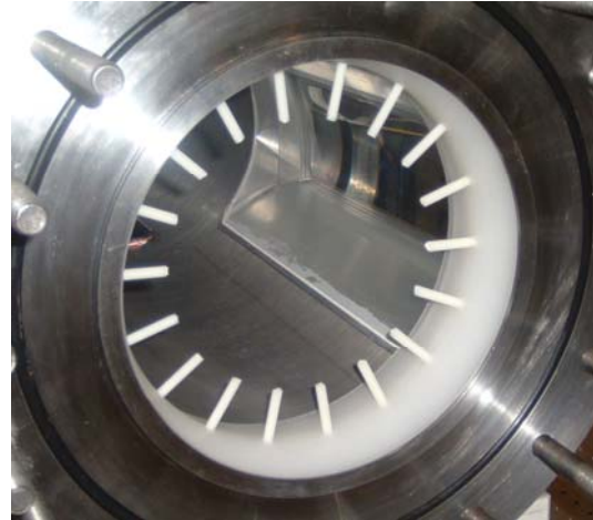
Figure 30: Picture of trip ring with 1.5 inch set screws at end of nozzle.
