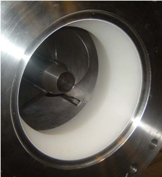
Figure 29: Picture of 0.75 inch maximum thickness compression ring in front of sting mount.
