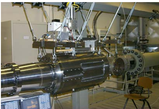
Figure 3 – Test and diffuser sections of the Purdue Mach-6 Quiet Flow Ludwieg Tube.
