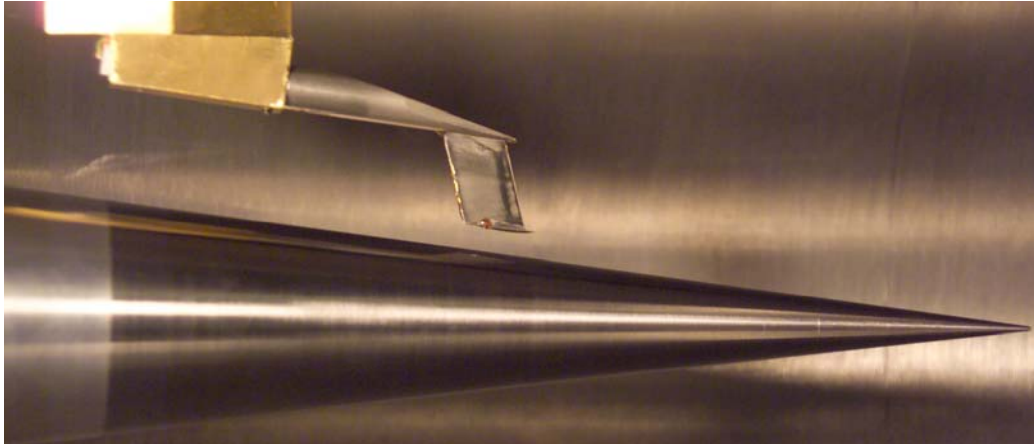
Figure 9 – Hot wire located near the cone wall in the test section of the Purdue Mach-6 Ludwieg Tube.
