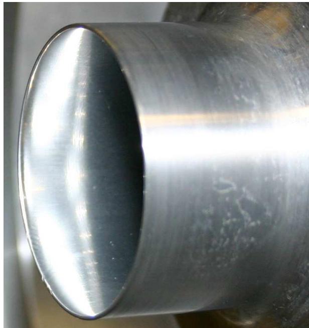
Figure 5: Polished throat with nicks on bleed lip at 7 o'clock
