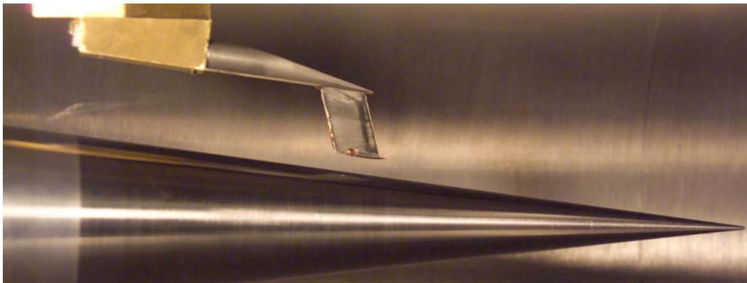
Figure 6 – Hot wire located near the cone wall in the test section of the Purdue Mach-6 Ludwieg Tube.
