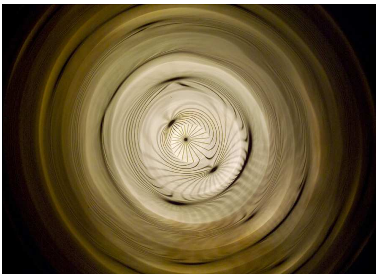
Figure 3: Photograph of Mach 6 nozzle looking upstream towards the throat showing some waviness
