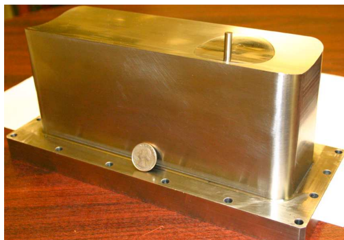
Figure 16: Roughness element with circular insert installed in forward window blank.
