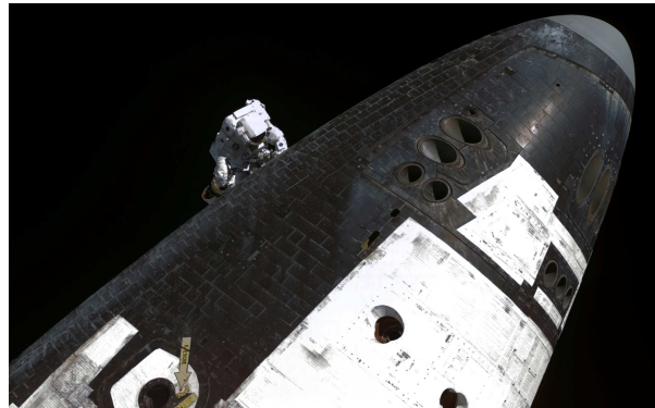
(b) Spacewalk to remove protruding gap filler. 11
