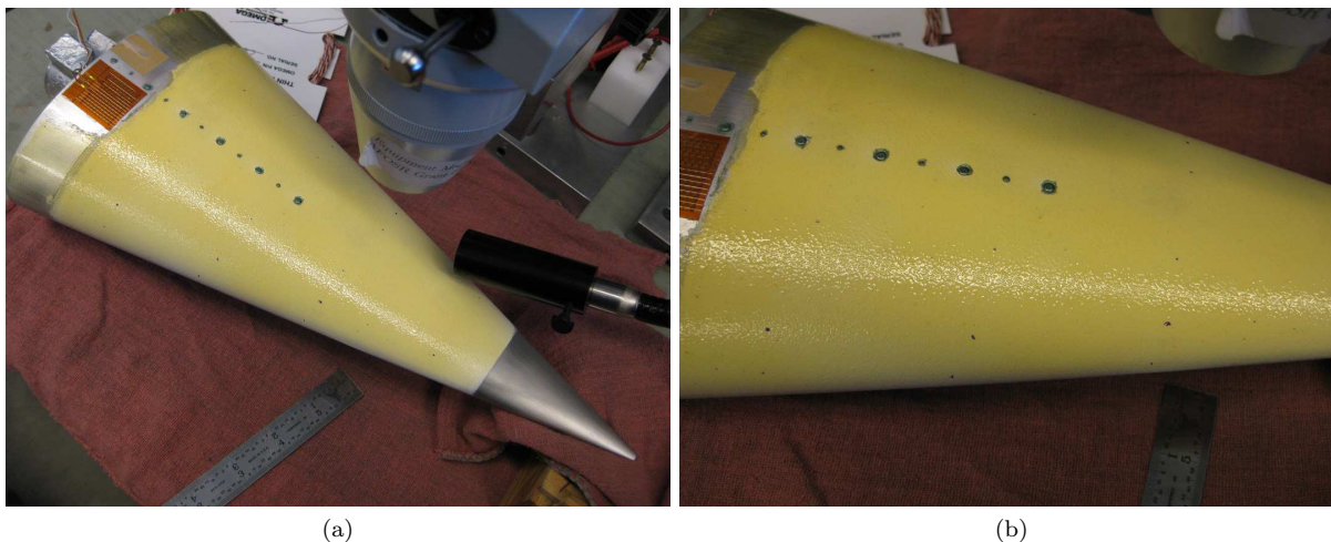
Figure 7: Photographs of first TSP application showing ‘orange-peel’ roughness
