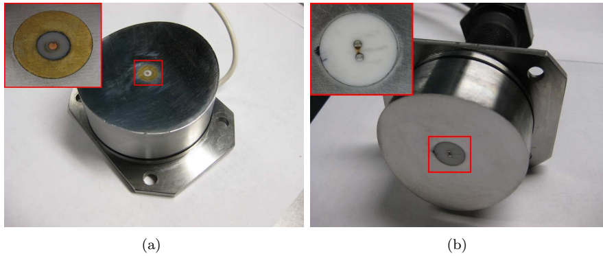
Figure 2. Electrodes (a) Glow-perturber; (b) Spark-perturber.
