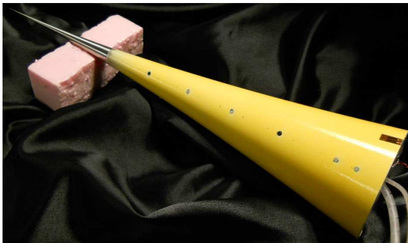
Figure 18. Compression cone model with 0.16-mm nosetip
