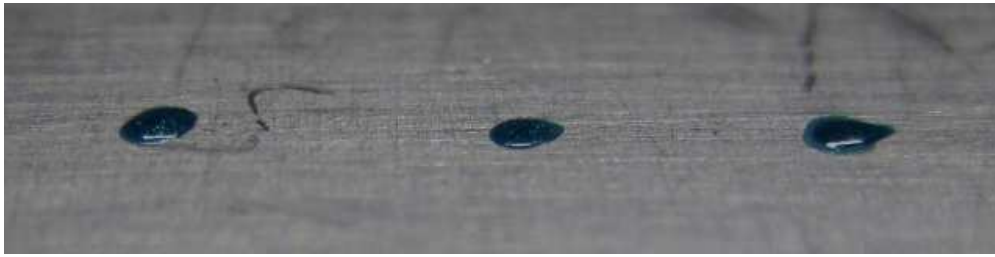
Figure 26. Photo of dots showing variation in shape for a fixed volume of 0.6 \mu\text{L} .
