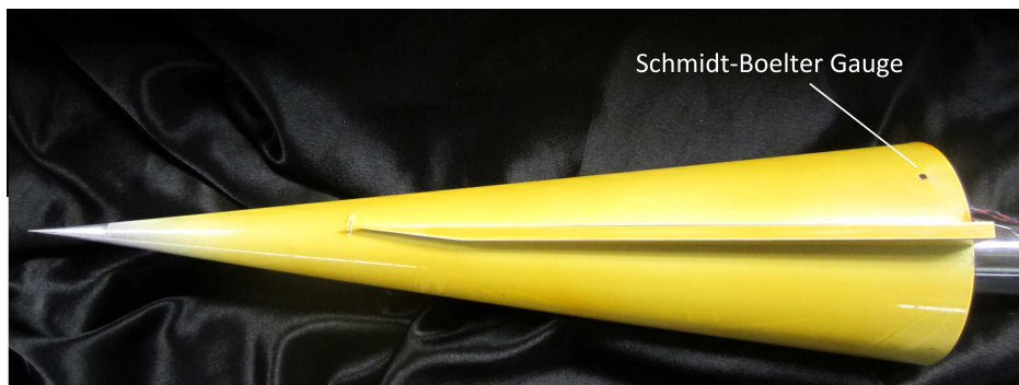
Figure 15. Modified Straight Cone Model.
