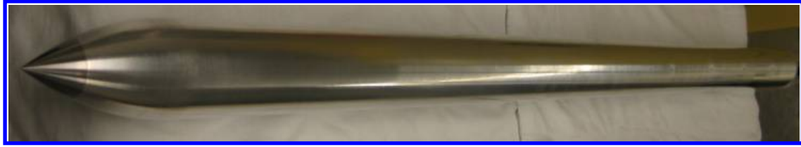
Figure 15. Picture of the Cone-Ogive-Cylinder being tested in the BAM6QT.
