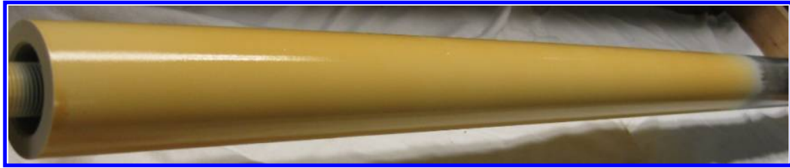
Figure 16. Picture of the Cone-Ogive-Cylinder after being painted with Temperature Sensitive Paint.
