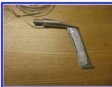
Figure 13. Pitot Probe with installed B-screen Kulite pressure transducer.
