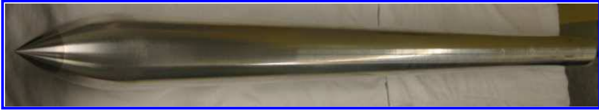
Figure 10. Picture of the cone-ogive-cylinder with the 30-degree nosetip.
