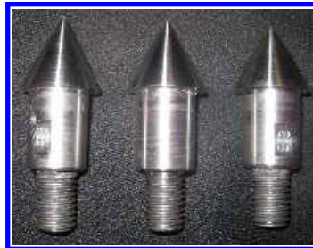
Figure 12. Picture of the cone-ogive-cylinder 28°, 30°, and 33° nosetips.
