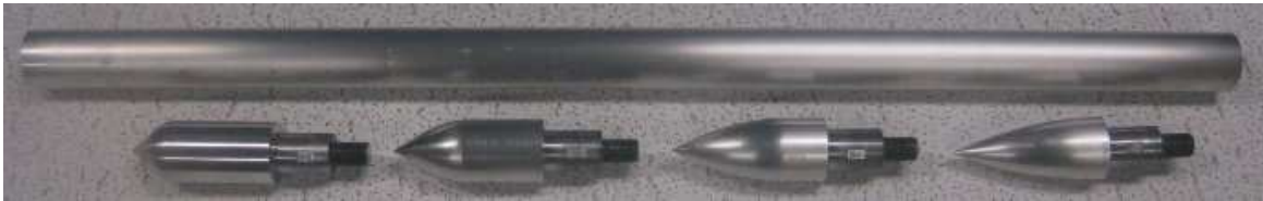
Figure 26. Picture of cone-ogive-cylinder model with interchangeable cone-ogive portions.
