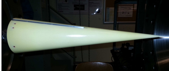
Figure 2. 7^\circ half-angle cone with temperature sensitive paint applied and no fin installed.
