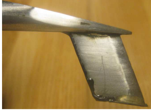
Figure 28. Picture of a hot-wire probe used in the BAM6QT.
