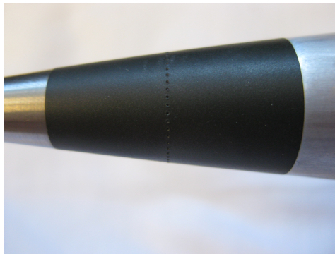
Figure 9. Torlon section and 50 roughness-elements (dimples).
