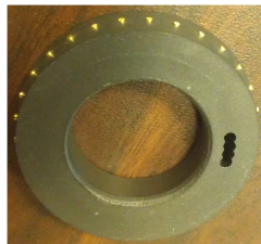
Figure 2. RIM roughness with brass rods of height = 381\ \mu\text{m} and diameter = 838\ \mu\text{m} .
