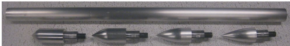
Figure 33. Photo of Cone-Ogive-Cylinder Model with Interchangeable Cone-Ogive Sections
