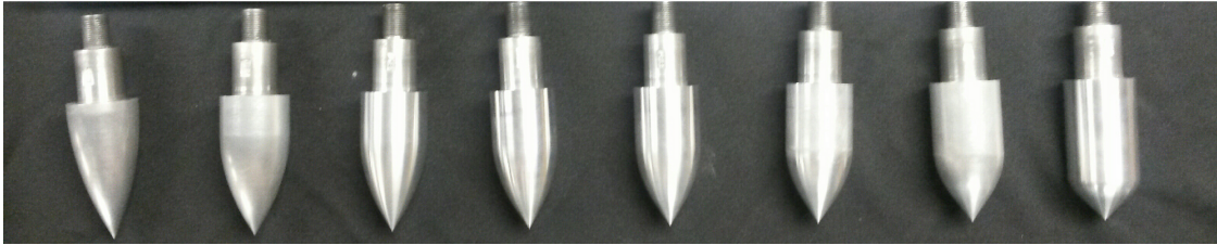
Figure 35. Picture of all eight interchangeable cone-ogive portions of the cone-ogive-cylinder model.
