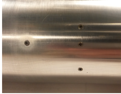
Figure 37. Picture of Kulite pressure transducers at x = 52 and 54 cm as well as two open sensor ports at x = 56 cm.
