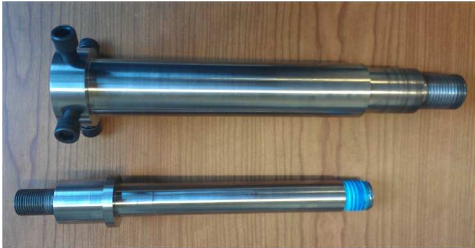
Figure 7. Photograph of adjustable angle-of-attack adapter. Metal rod in lower half of photograph holds the model and inserted into upper piece.
