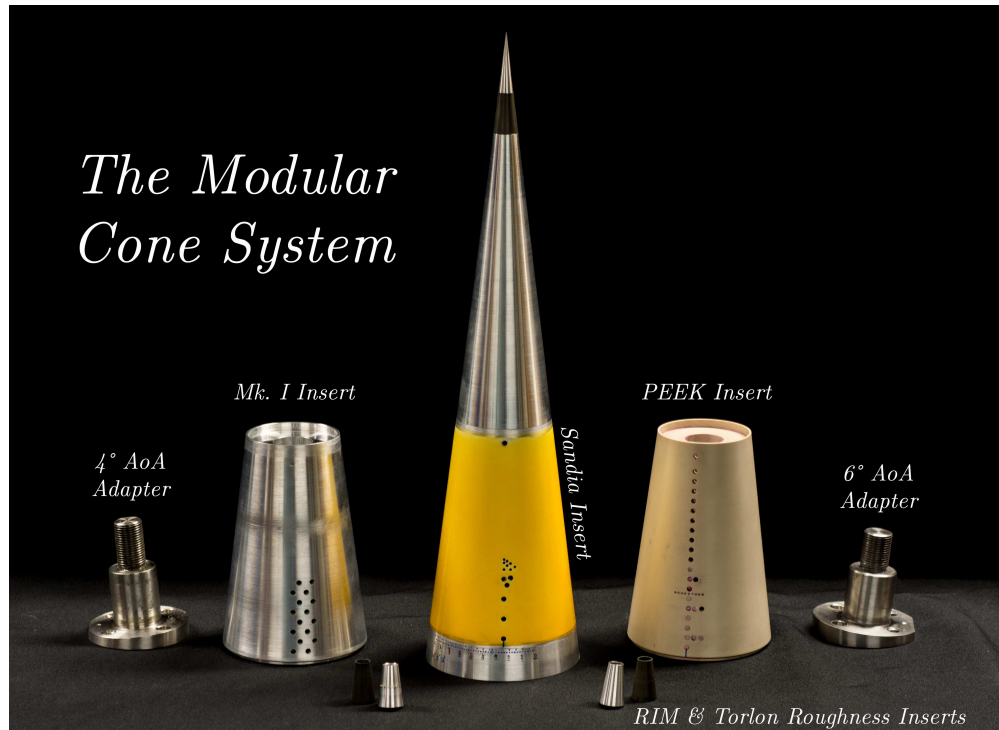
Figure 15. A photograph of the Modular Cone System, including the three available sensor inserts and four of the many roughness inserts.
