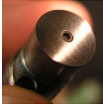
Figure 3.15. Mic-062 A-screen installed in individual insert
