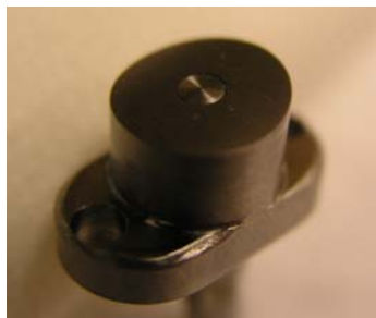
Figure 3.16. PCB105 installed in individual insert
