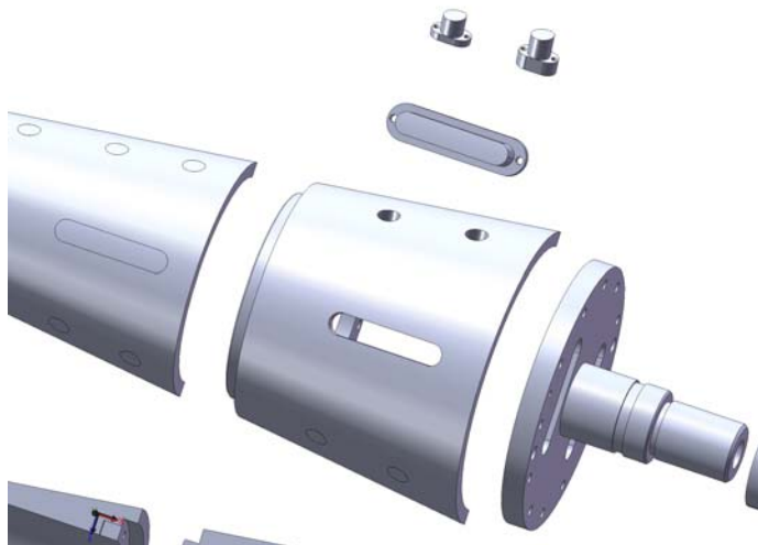
Figure 3.12. Two individual inserts and one axial insert removed from model
