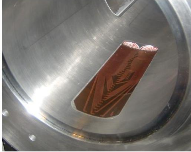
Figure 3.2. Hot-film array at downstream end of nozzle (Fig. 2.14 from Ref. [10])
