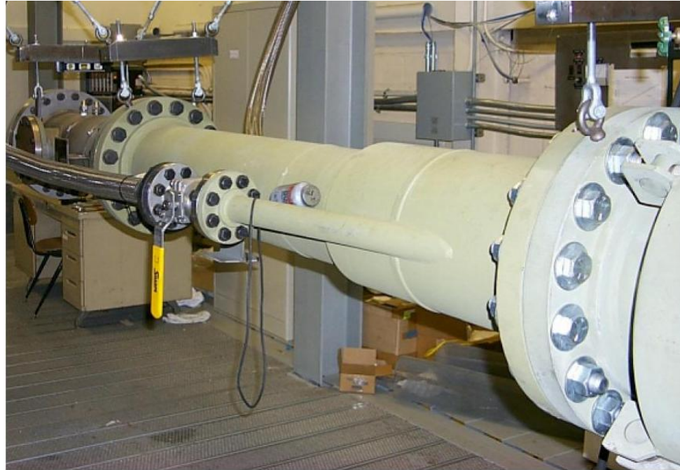
Figure 2.3. Original sting-support and diffuser sections
