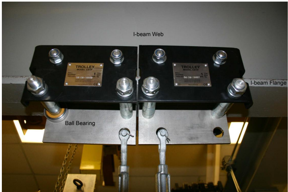
Figure D.11. Modified trolleys at the junction between the adapter flange and sting-support section
