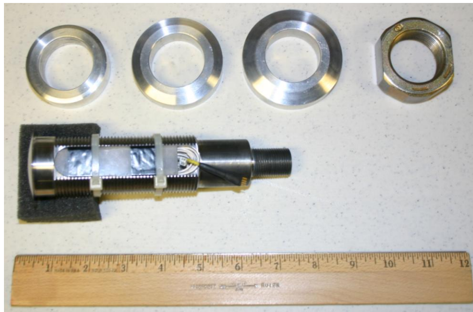
Figure 2.7. Sphere-cone model used on blockage tests (top row left to right: 2.25-inch disk, 2.5-inch disk, 2.75-inch disk, and retaining nut; middle row: 2-inch sphere-cone model)
