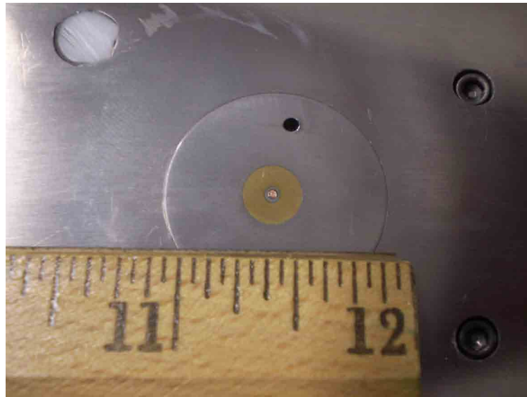
Figure 5.14: Glow perturber as installed
