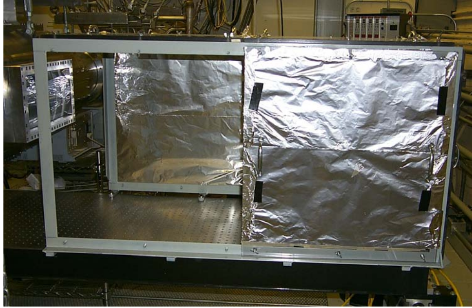
Figure 2.3. Assembly of the Lexan window enclosure.
