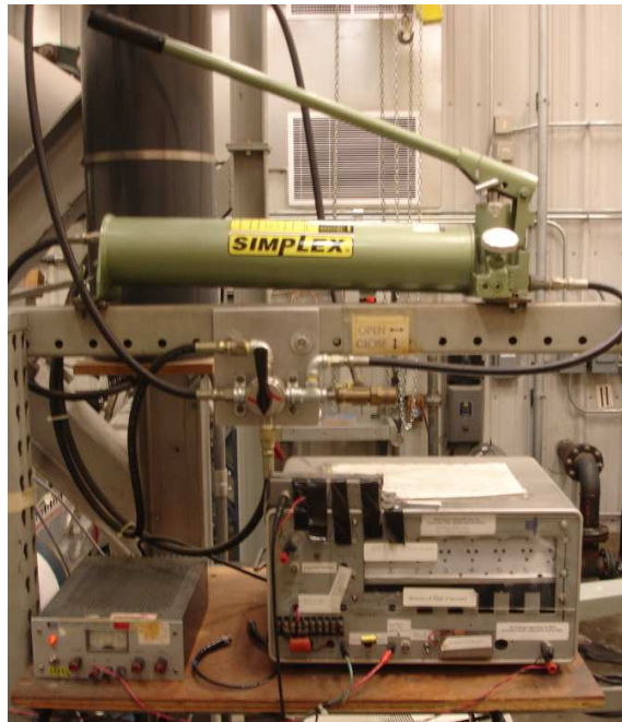
Figure B.9: PQFLT facility, sliding sleeve controls and diaphragm burst electronics
