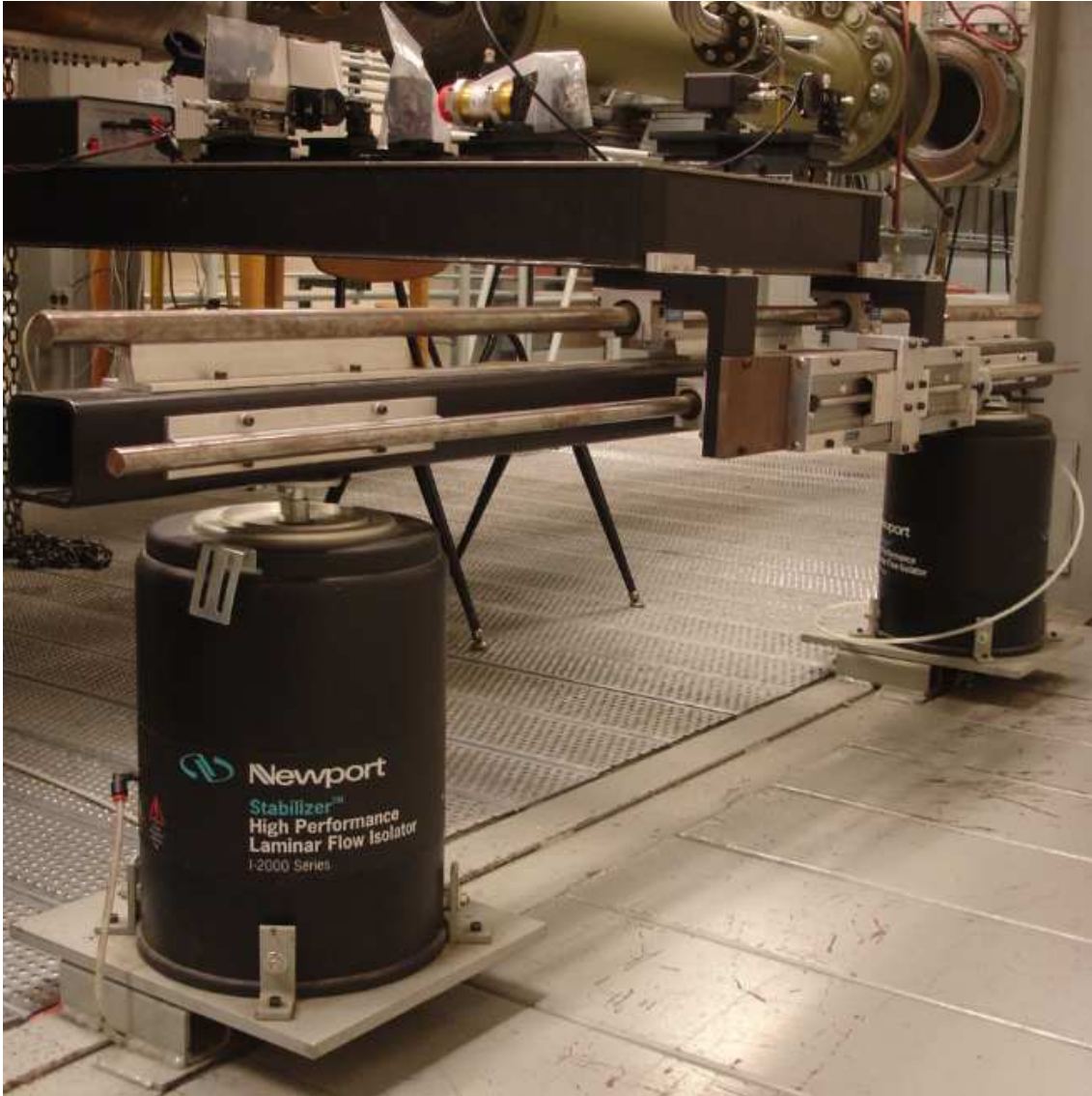
Figure B.20: BAM6QT facility, vibration control system
