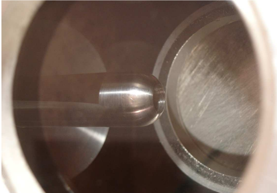
Figure B.28: Forward-facing cavity model inside PQFLT
