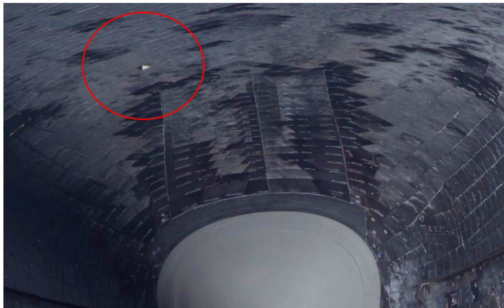
Figure 1.2. Example of an isolated roughness: protruding gap filler on Space Shuttle Mission STS-114, removed by astronaut in orbit [27].
