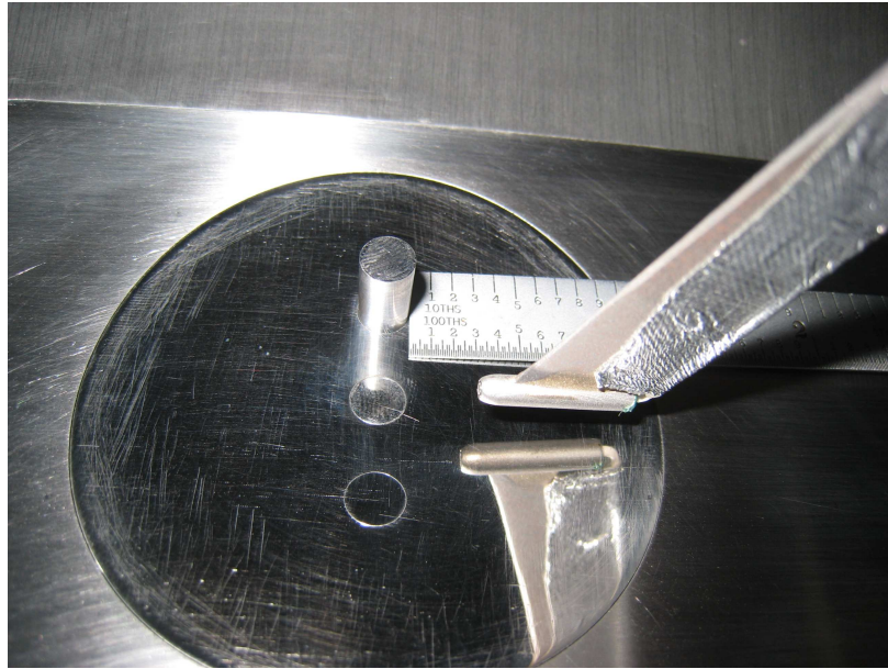
Figure 5.2. Example of measuring off of the roughness centerline. Flow is from left to right. A scale with tenths and hundredths of inches is shown.
