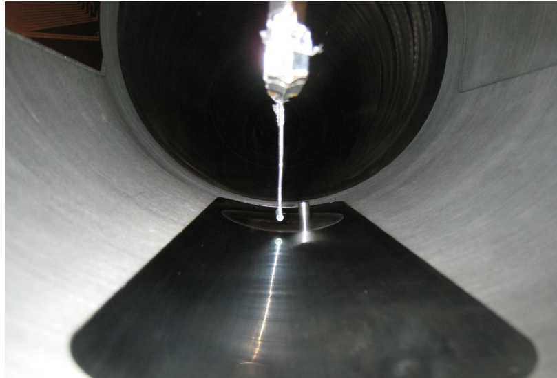
Figure 5.3. View of pitot probe and roughness, looking upstream.
