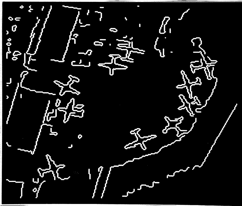
Figure 5.21 Edges of airplanes image detected using a priori information about the features of interest. Top: CCF approach. Bottom: ACF approach.
