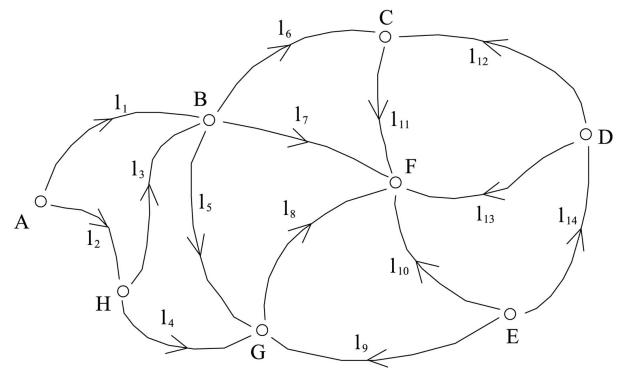
Adjust the level network by least squares using the method of observations only. Arrows point up hill as indicated by the observations. Use appropriate weights as indicated by the sigmas.
