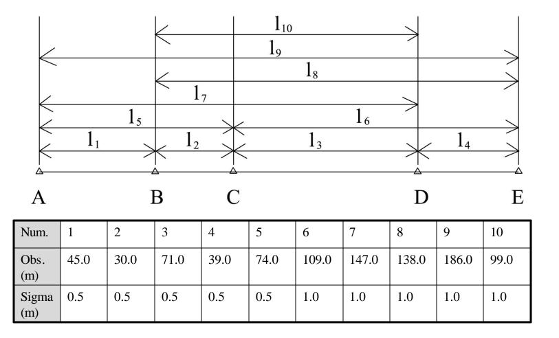
The model is 4 collinear distances. Adjust by least squares using the method of observations only. Use weights according to the given sigmas.
