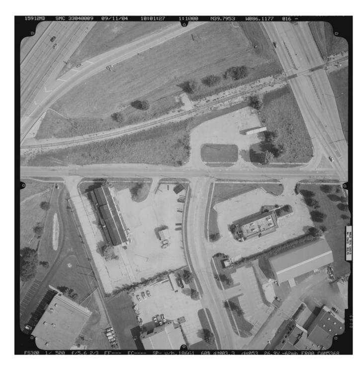
INDOT / Woolpert / Spectrum I-70 Imagery, Camera RC30, Alt(amt) 500 ft., Scale 1:1000, Scanned 14um, GSD 1.5cm or 0.6 in
