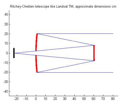
The primary and secondary surfaces are defined by the following equation for a hyperbola which is presented in the form used for optical design, R being the radius of curvature at the origin, K being the conic constant (units are cm). Original ray at y=20.3
