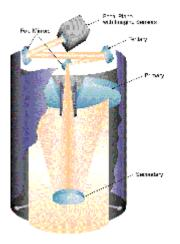
Alignment error of each curved mirror is so small it must be measured in wavelengths of light. "It's equivalent to placing a human hair under one end of a 20-foot plank of wood," says Lloyd. Specifically, the mirrors must not deviate by more than a handful of arc seconds during the rock-and-roll ride into orbit, when settling into zero gravity, across 50° temperature swings inside the spacecraft, or resulting from vibrations caused by spacecraft maneuvering and telescope pointing.
