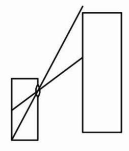
A solution: shift the lens up parallel to the image plane, i.e. detector and lens are no longer "lined up", but you now get the coverage you want plus the object lines remain parallel
