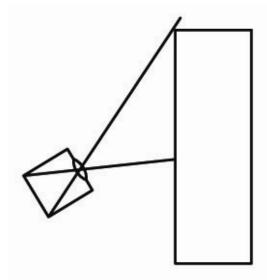
Image plane not parallel to the object plane causes the convergence of lines which is characteristic of perspective projection
