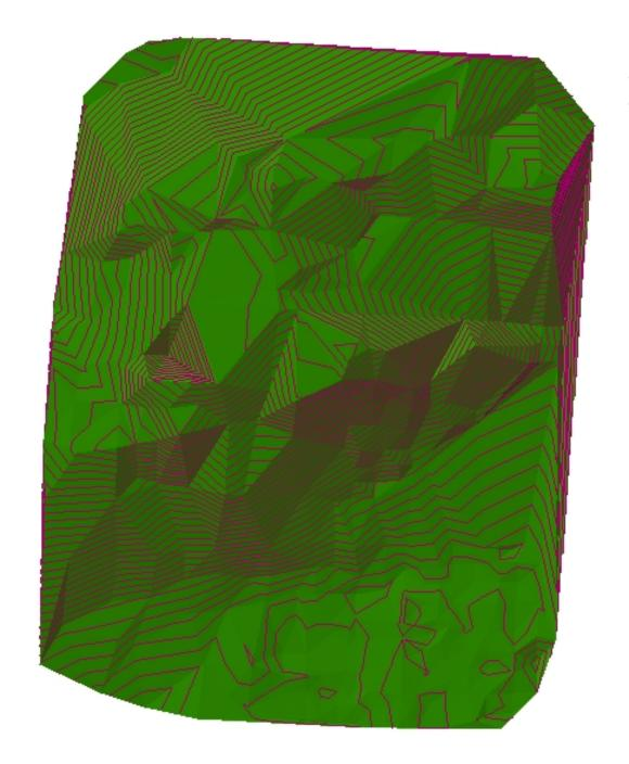
Contour plot from ArcGIS TIN utility – only spot elevations
