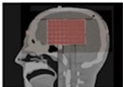
Assess TPS image fusion and image transfer accuracy with multi-modality imaging inserts for CT, MRI and PET
