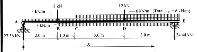
The equation for the **bending moment** at x is:
