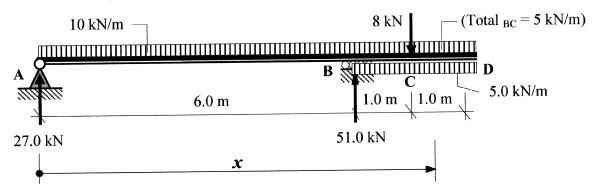
The equation for the **bending moment** at x is:
