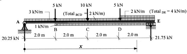
The equation for the **bending moment** at x is:
