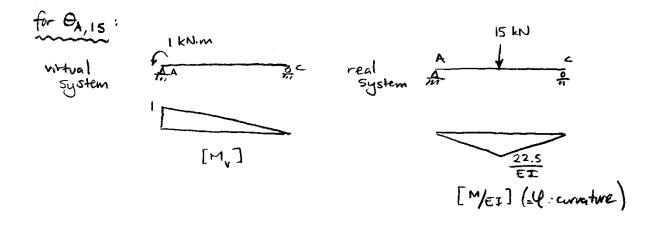
Equating external virtual work to internal virtual strain energy
