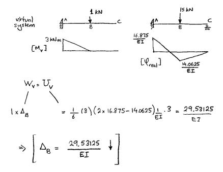
Same result as before. The released redundant force (reaction at *C*) does not do any external virtual work or cause any internal virtual strain energy because the vertical displacement at *C* in the real system is zero.
