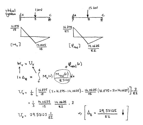
b) Virtual system is a simply supported beam with a unit vertical load applied at B.
