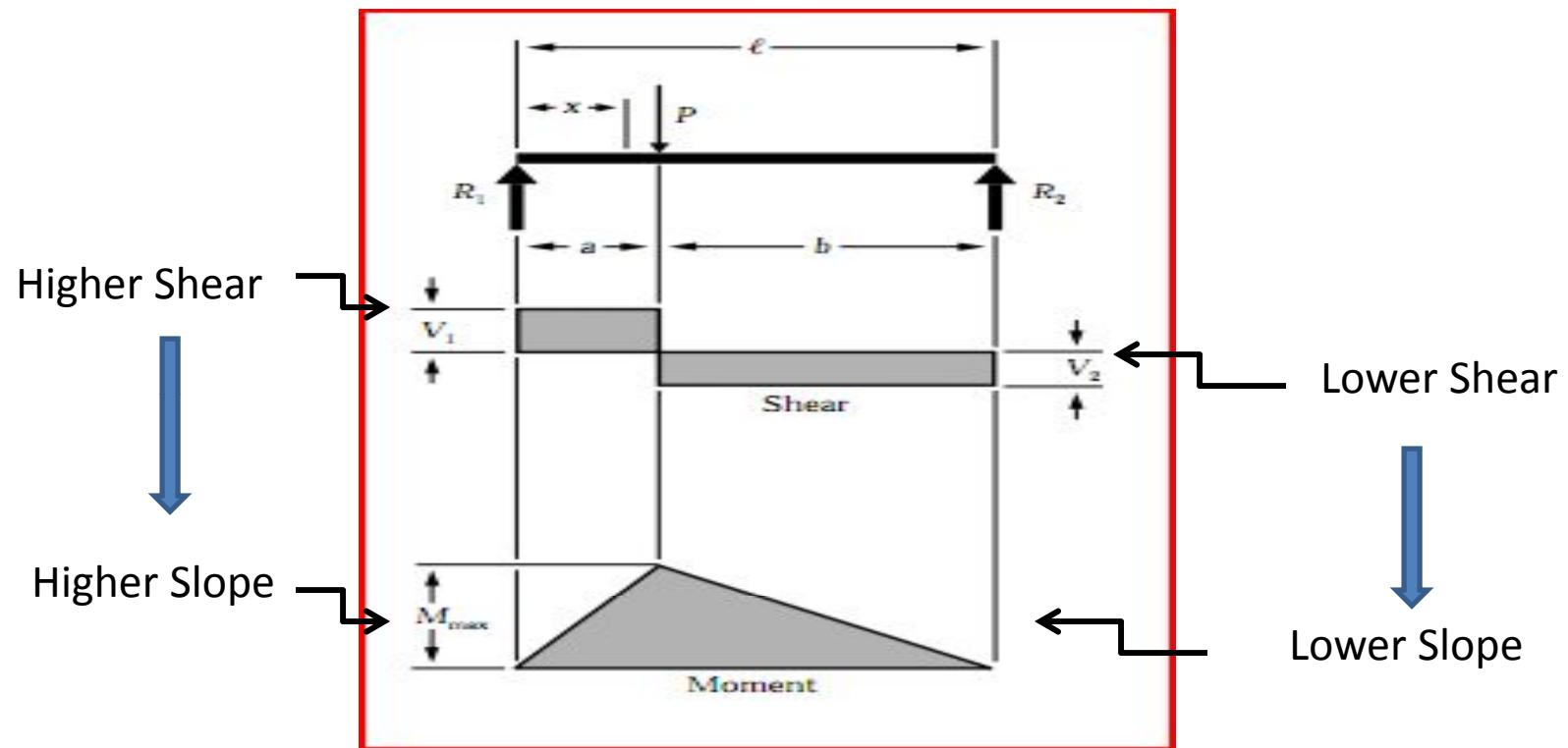
Shear = (negative)Slope of Bending moment (i.e.  $V = dM/dx$ )
