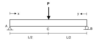
Let's consider flexural behavior only. To find the total strain energy, we need to find the internal bending moment over the member and the corresponding curvature. To be able to make use of Castigliano's 2<sup>nd</sup> theorem, we need to express the internal strain energy in terms of P, the load.
